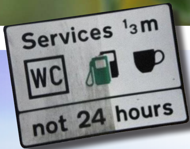
ACTIVA effect in half a traffic sign, after several years of weathering
